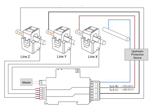
1P+N System Wiring up to 3 Branch Circuits
